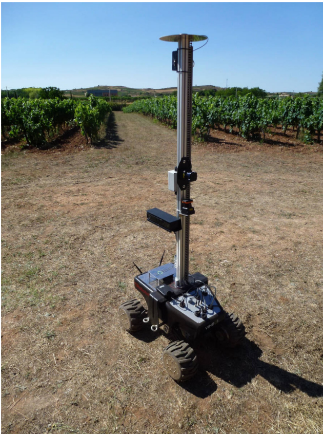
Fig. 11. The VINEBOT is responsible for vineyard monitoring and management.
