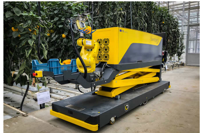
Fig. 9. The SWEEPER is designed to harvest peppers in a greenhouse.
