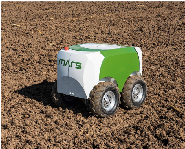
Fig. 7. UGV from project MARS is able to work in swarms.
