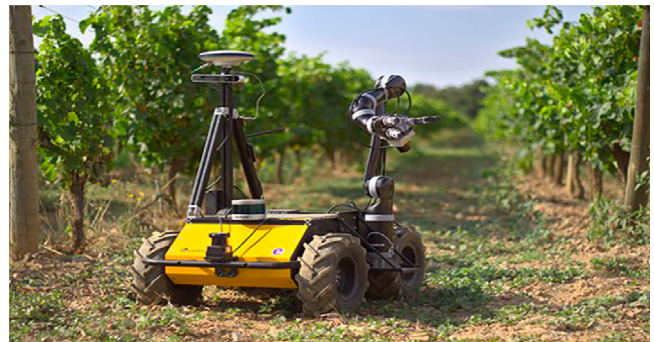
Fig. 8. UGV from subproject GRAPE suitable to operate in vineyards.
