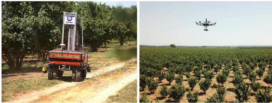
Fig. 13. The developed UAV and UGV from PANtHEOn project are able to collect information at the resolution of a single plant.
