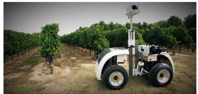
Fig. 10. The VINEROBOT is capable of monitoring grape growth.
